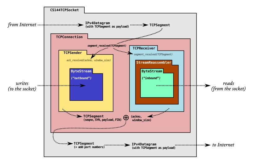
Figure 1: The arrangement of modules and dataflow in your TCP implementation. The ByteStream was Lab 0. The job of TCP is to convey two ByteStreams (one in each direction) over an unreliable datagram network, so that bytes written to the socket on one side of the connection emerge as bytes that can be read at the peer, and vice versa. Lab 1 is the StreamReassembler, and in Labs 2, 3, and 4 you'll implement the TCPReceiver, TCPSender, and then the TCPConnection to tie it all together.
