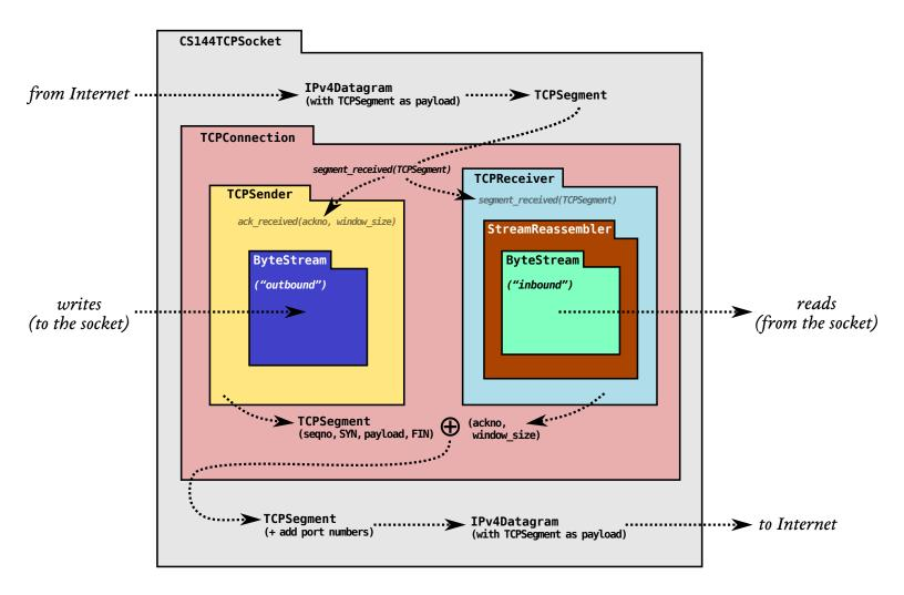
Figure 1: The arrangement of modules and dataflow in your TCP implementation.
