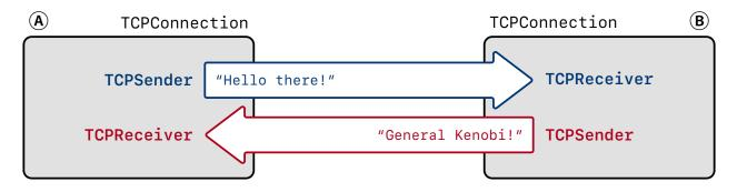
The two parties ("A" and "B" in the above diagram) are called the "endpoints" of the connection, or the "peers." Your TCPConnection acts as *one* of the peers. It's responsible for receiving and sending segments, making sure the sender and receiver are informed about and have a chance to contribute to *the fields they care about* for incoming and outgoing segments.
