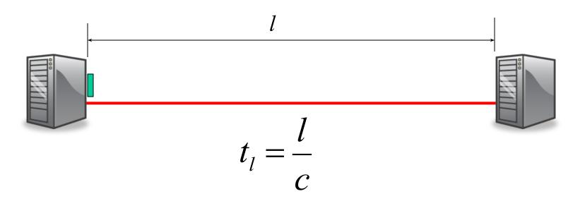
Example: A bit takes 5ms to travel 1,000km in an optical fiber with propagation speed 2 x 10<sup>8</sup> m/s.
